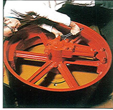
Frang iron protection is provided by a spring loaded safety device.
