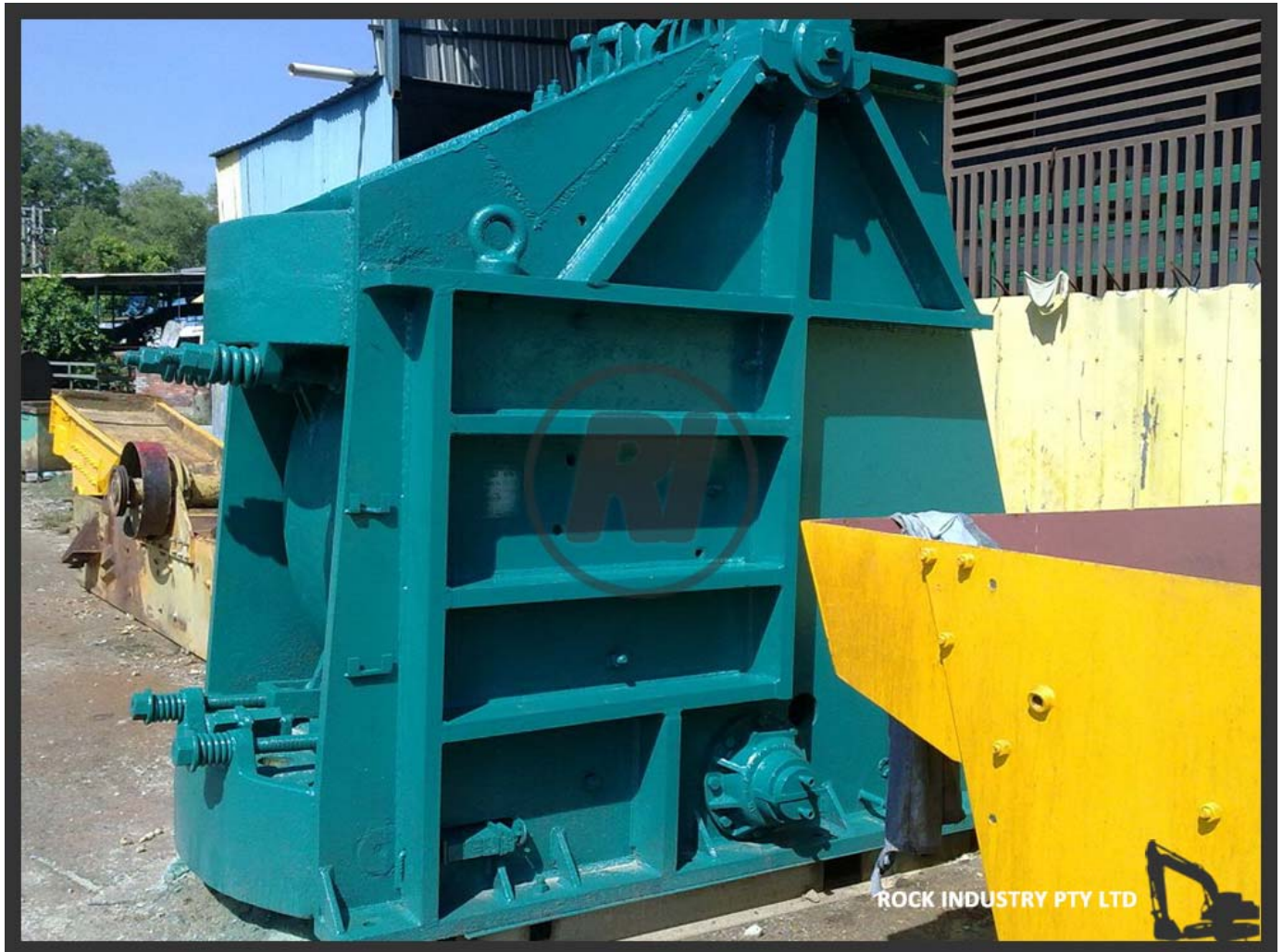
BROWN LENOX KUE KEN Model 120S – 42" x 36" Double Toggle Jaw Crusher.
