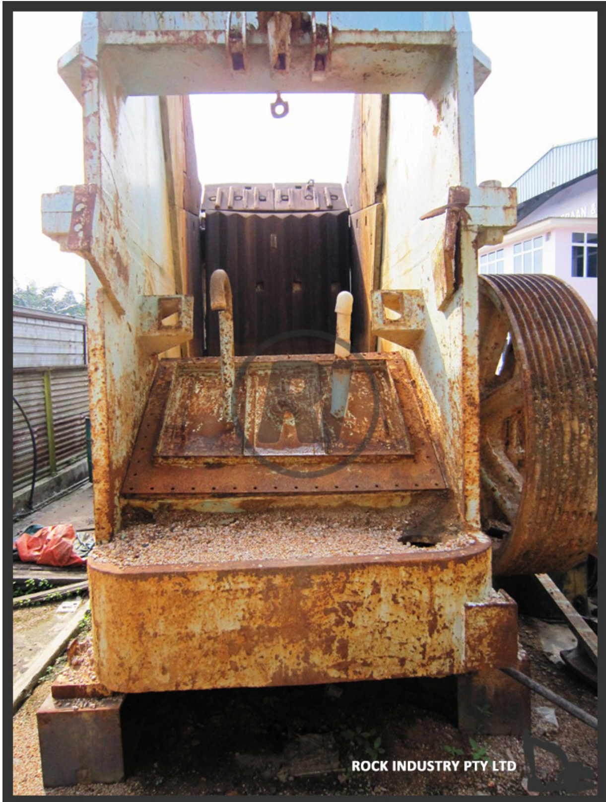
BROWN LENOX KUE KEN Model 160 – 48" x 42" Double Toggle Jaw Crusher.
