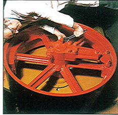
Flange iron protection is provided by a spring loaded safety device.
