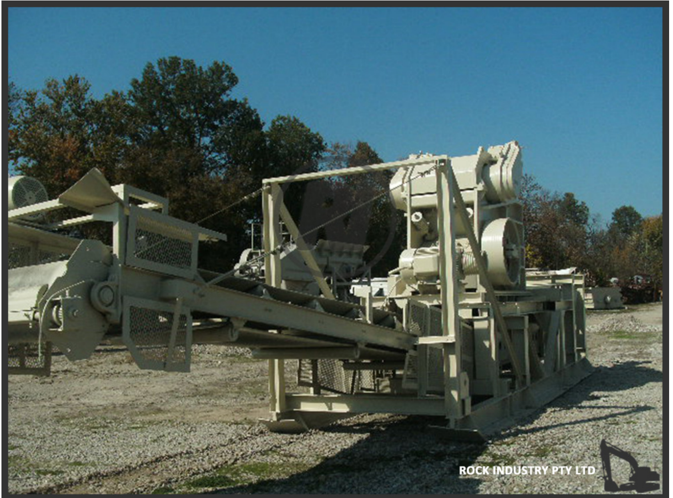
KUE KEN KK126 – 42" x 36" Jaw Crusher. LIPPMANN 20' Vibrating Feeder SKID FRAME, MOTORS and Discharge Conveyor.
